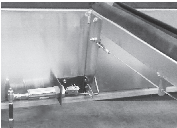
FIGURE 8 ACTUATOR AND LATCH MECHANISM 010290
