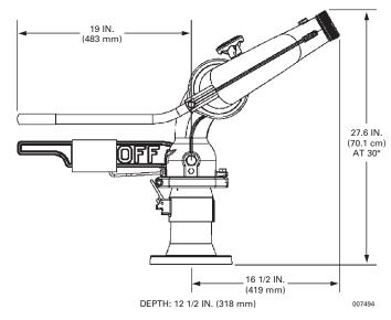
The Protector Station Monitor is recommended for use with ANSUL® Master Stream nozzles and ANSUL Master Foam nozzles.
